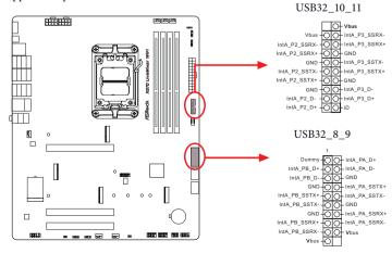
Front Panel Type C USB 3.2 Gen2x2 Header (20-pin USB32\_TC2) (see p.7, No. 13)
