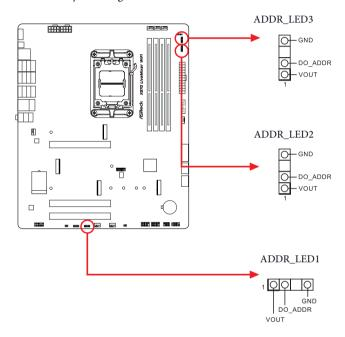
Connect your Addressable RGB LED strips to the Addressable LED Headers (ADDR\_LED1 / ADDR\_LED2 / ADDR\_LED3) on the motherboard.
