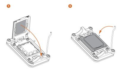
Make sure the CPU is aligned with the socket before locking it into place.
