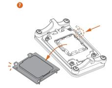
Make sure the black cover plate is always in place until it pops off when closing the socket lever.
